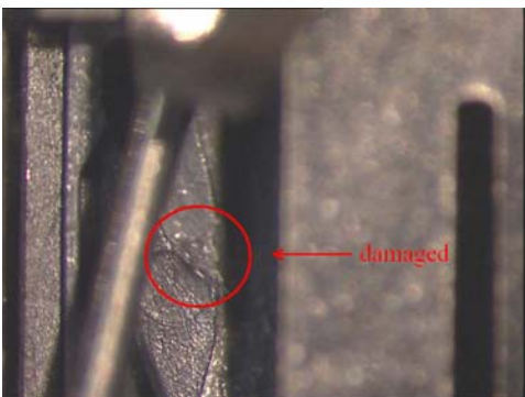
Lock mechanism damaged
